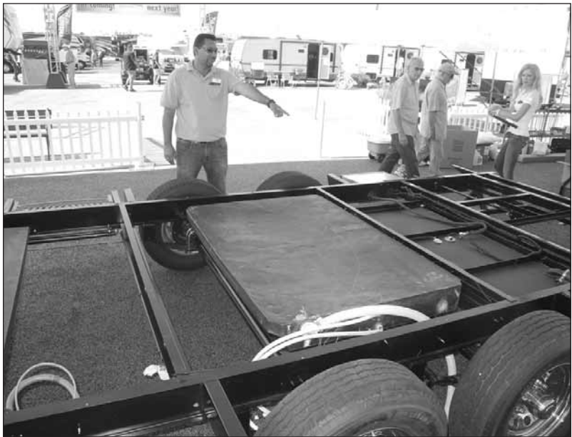
BUILDING A TRAILER AT THE SHOW – Pablo Carmona, President and CEO of Genesis Supreme in Perris, shows off the frame on opening day at the California RV Show at Fairplex – with water and gas tanks already installed – that will be used to assemble the first-ever complete trailer built on site at the show. The finished product will be a 19-foot toy hauler that will sell for about $20,000. Carmona, who has worked in the industry for the past 25 years, opened Genesis Supreme three years ago and has grown to 70 employees.
