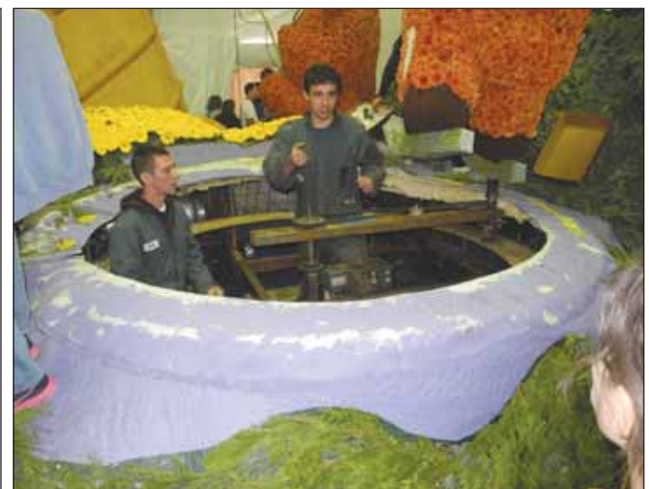
Students explain the float's hidden animation controls to a visitor. Moments later, the hatch cover -- consisting of a layer of plywood and a steel plate -- was lifted into place.
