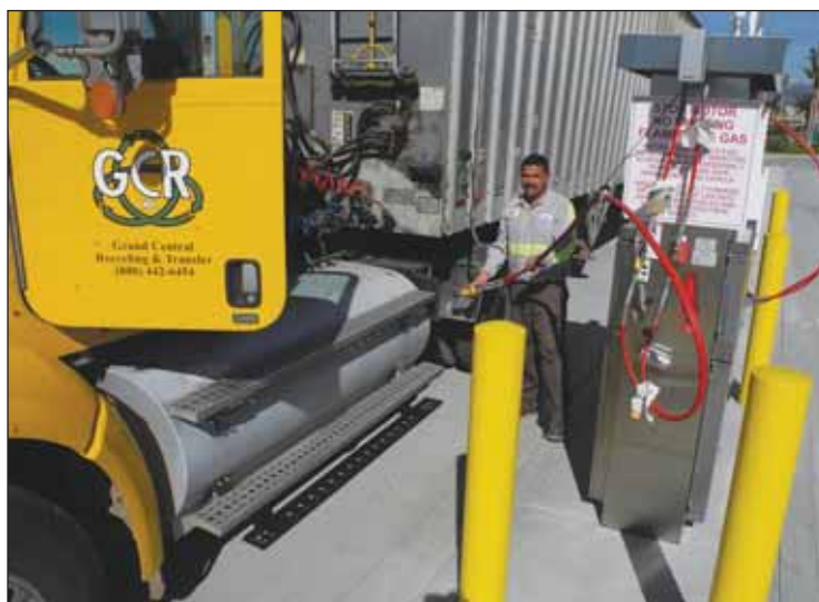
Driver Manuel Madueno, operator of a vehicle from Grand Central Recycling & Transfer, part of the Valley Vista Services family of companies, fills his vehicle with compressed natural gas at the new dispensing facility at the Pomona Valley Transfer Station in Pomona.
