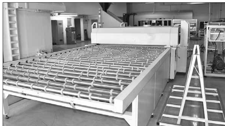
Solar panels will roll out of this laminator where the layers are sealed together before framing.
