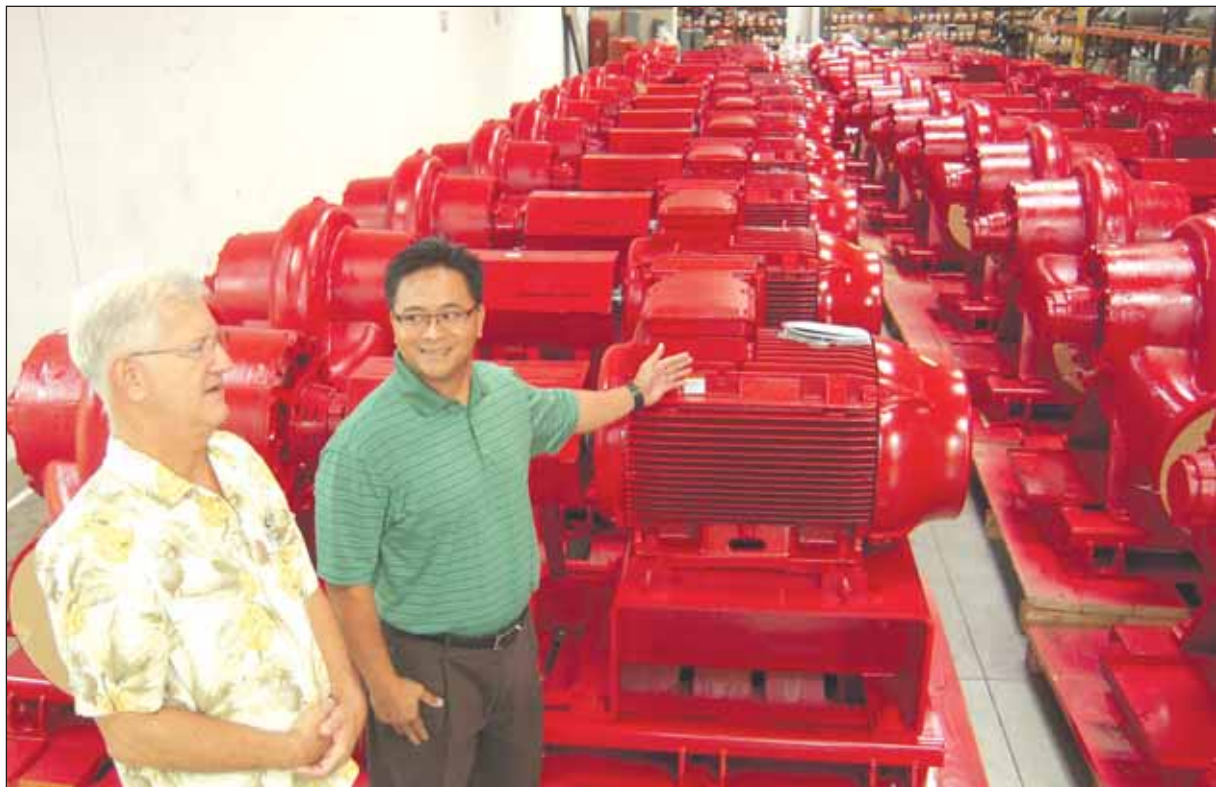
AIR CONDITIONING PUMPS HEADING FOR LAX -- Dawson Co. President and CEO Ric Serafin, at right, shows La Nueva Voz Publisher Jeff Schenkel a total of 52 Bell & Gossett centrifugal pumps for air conditioning systems during a tour last week of his 33,400 square foot facility in Pomona. The pumps, ranging in size from 100 to 200 horsepower, will become part of a new air conditioning system for the central utility plant at Los Angeles International Airport. Dawson Co. also is working on a thermal energy storage system at Loma Linda University and Medical Center. Dawson Co., which has 30 employees in Pomona, four in San Diego and one in a satellite office in San Luis Obispo, was named the Pomona Chamber of Commerce "Employer of the Year" at the Pomona Chamber awards banquet in June. The company moved to Pomona three years ago but has been in business since 1948. It serves as manufacturers' representatives and distributors of residential, commercial and industrial plumbing, heating and cooling equipment.
