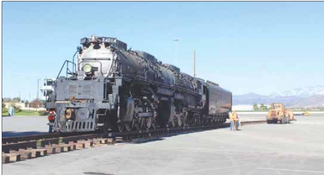
'BIG BOY' WAVES BIG GOODBYE TO FAIRPLEX -- Big Boy UP4014, one of the largest steam locomotives ever built, is making tracks for Wyoming from its home for the last 50 years at the RailGiants Train Museum at Pomona's Fairplex. The train is heading to Union Pacific Railroad's heritage operations to be restored to operating condition. Pictured is part of the special new temporary track that was laid across the Fairplex parking lot to connect the train from the museum to the Metrolink tracks at Arrow Highway. The train was to be hauled to Covina where it was to be transferred to Union Pacific tracks, and then driven to Union Pacific's Colton plant for a brief bit of restoration before heading to Cheyenne, Wyoming some 1,260 miles away. The restoration project is expected to take several years. Pictured is the tractor that was used to tow the train across the temporary tracks.
